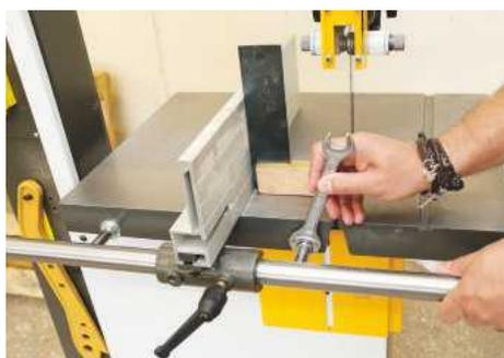
▲ The deep fence is easily set for square by minor adjustments to the running bar
